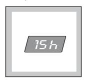
The delay time is displayed for 3 seconds, then the duration of the selected programme reappears. After you have pressed the "**Start/Pause**" button, the countdown begins, and the delay time value decreases by one unit every hour and then, when 2 hours remain, the time decreases in 30 minute intervals. You can delay the start of the selected programme by up to 23 hours in one hour intervals.
